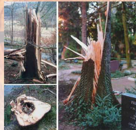
Figure 1. Two of many examples of broken conifer trees (in these cases, of Picea abies ). The tree on the left had a small defect in the center at the stem base with t/R \approx 1/2 but broke on a height where t/R \approx 4/5 ( > 1/3 ). The tree on the right was fully intact ( t/R = 1 ) and broke in a combination of torsional and dynamic loading in a thunderstorm.
